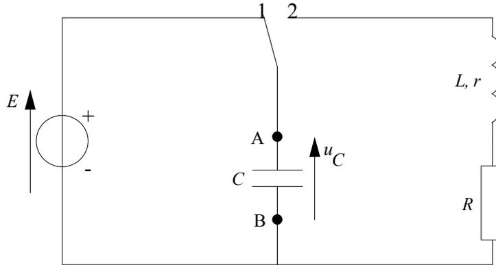
$R = 20 \Omega, 39 \Omega, 150 \Omega, 390 \Omega, 1000 \Omega$  ou  $3000 \Omega$ ;  $L = 1 \text{ H}$  variable;  $C = 5 \mu\text{F}, 10 \mu\text{F}$  ou  $15 \mu\text{F}$ .
